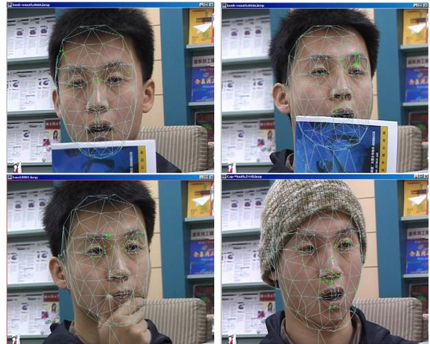
Figure 8: Tracking results under occlusion with certain illumination variation.
