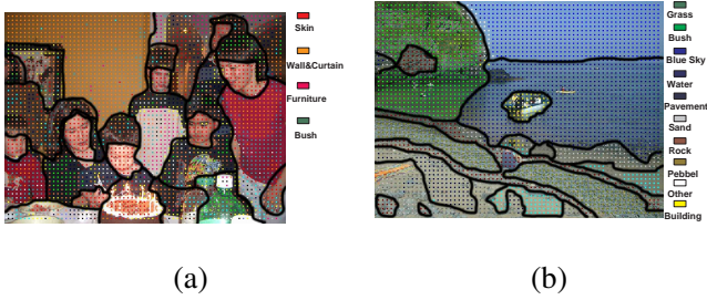
Figure 3.4: (a) The local patch material labeling results of an indoor photo. (b) The local patch material labeling results of an outdoor photo. Loopy belief propagation is used for enhancement. The colored dots represent the material label and the boundaries are manually overlaid for illustration purpose only.
