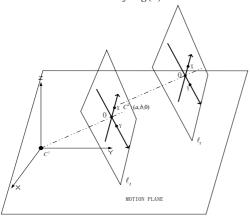
Fig 3: Different locations of camera under a pure tanslation on the motion plane.
