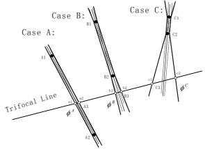
Fig 7: the projection from 2D image points to 1D image points. (• is the distribution area of the random uncertainty for 2D image points. The black lines are the bound of uncertainty for the 2D-1D projection. Here, A, B, C are three cases of 2D to 1D projections.)
