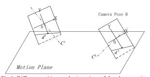
Fig 1: Different positions and orientations of the planar motion cameras.  $(C^1, C^2)$  are the optical centers of cameras,  $OC^1, OC^2$  are the optical axes of cameras and XOY is the coordinates in
