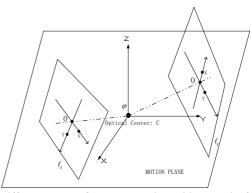
Fig 4: Different poses of camera rotating with normal of the motion plane.
